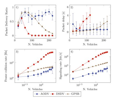
Fig. 3. Performances of the selected routing algorithms (AODV, DSDV, and GPSR) for a 300 kbit/s data flow, ignoring the shadowing effects caused by the buildings.
