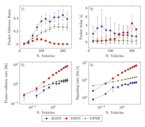
Fig. 4. Performances of the selected routing algorithms (AODV, DSDV, and GPSR) for a 300 kbit/s data flow, considering the shadowing effects caused by the buildings.
