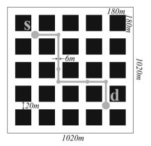
Fig. 2. Representation of the simulated Mahattan scenario. The larger gray nodes are the fixed source and destination vehicles, while the smaller nodes are the intermediate relays selected by the routing protocol. We observe an example of an established unicast route over 6 hops.
