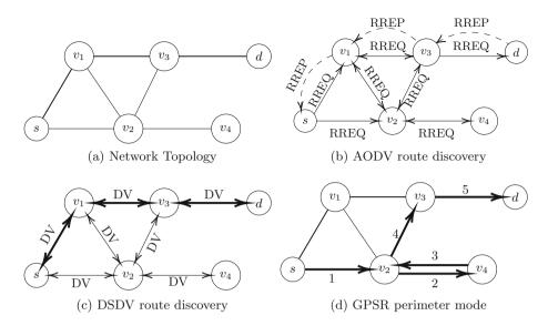
**Fig. 1.** Features of AODV, DSDV, and GPSR. On (a) an example of VANET connectivity graph, with a source vehicle s and a destination vehicle d, (b) illustrates the AODV's route discovery process, (c) shows the DSDV's distance vector broadcasting, with the computed route in bold, and (d) shows the route of a packet in GPSR perimeter mode to bypass a void area, where the numbers are the sequence of links on which the data packet is forwarded.
