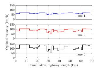
Figure 7: Mean vehicle velocity  $v_{ik}$  for lane i = 1, 2, 3 as a function of the distance on GRA starting from exit k = 1  $(n = 10, D_{0q} = 3 \text{ min})$ .
