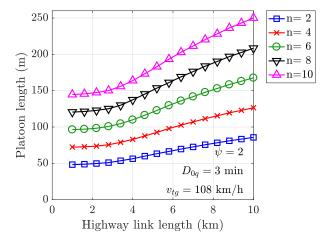
Figure 4: Platoon length with respect to the highway link length under the mean delay constraint  $D_{0q} + l/v_{tg}$  and different values of
