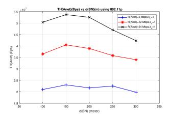
Figure 15: Maximum delay-capped  $TH_{\rm Anet,I}$  (bit/s) and  $PDR \ge 0.95$  vs  $d_{\rm BN}$  (m) for IEEE 802.11p Anet
