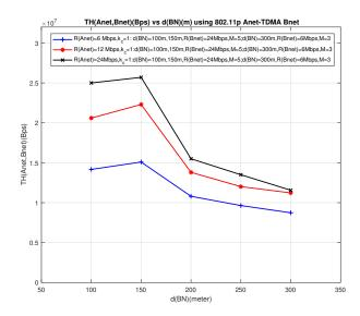
Figure 16: Delay-capped  $TH_{\rm Anet,Bnet}$  (bit/s) vs  $d_{\rm BN}$  (m) for IEEE 802.11p Anet-TDMA Bnet
