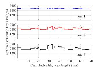
Figure 6: Mean link vehicular flow rates  $\phi_{ik}$  for lane i=1,2,3 as a function of the distance from exit k=1 on GRA  $(n=10,D_{0\mathrm{q}}=3\,\mathrm{min})$ .
