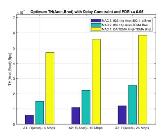
Figure 18: Comparison Delay-capped  $TH_{\rm Anet,Bnet}$  (Mbit/s) vs  $R_{\rm Anet}$  (Mbit/s) for N=250. Bar explanation: (A1/A2/A3,MAC3):  $R_{\rm Anet}=R_{\rm Bnet}$ ; (A1/A2/A3,MAC2):  $R_{\rm Bnet}=24\,{\rm Mbit/s},~M=5,~d_{\rm BN}=100\,{\rm m};$  (A1/A2,MAC1):  $k_c=2,~R_{\rm Bnet}=24\,{\rm Mbit/s},~M=5,~d_{\rm BN}=100\,{\rm m};$  (A3,MAC1):  $k_c=3,~R_{\rm Bnet}=24\,{\rm Mbit/s},~M=5,~d_{\rm BN}=100\,{\rm m};$
