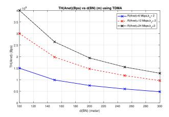
Figure 12: Aggregate Anet Throughput  $TH_{\rm Anet,I}$  (bit/s) vs  $d_{\rm BN}$  (m) using DA/TDMA,  $l=5\,{\rm km}$
