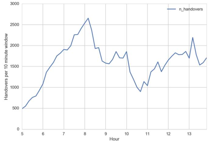
Fig. 4: Simulated mobile network handovers per 10 minute window
