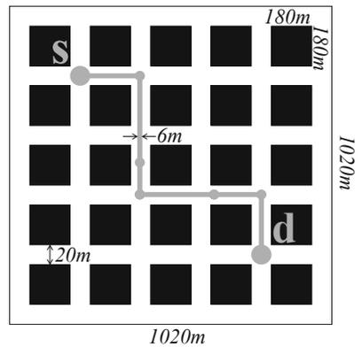
**Fig. 2.** Representation of the simulated Manhattan scenario. The larger gray nodes are the fixed source and destination vehicles, while the smaller nodes are the intermediate relays selected by the routing protocol. We observe an example of an established unicast route over 6 hops.
