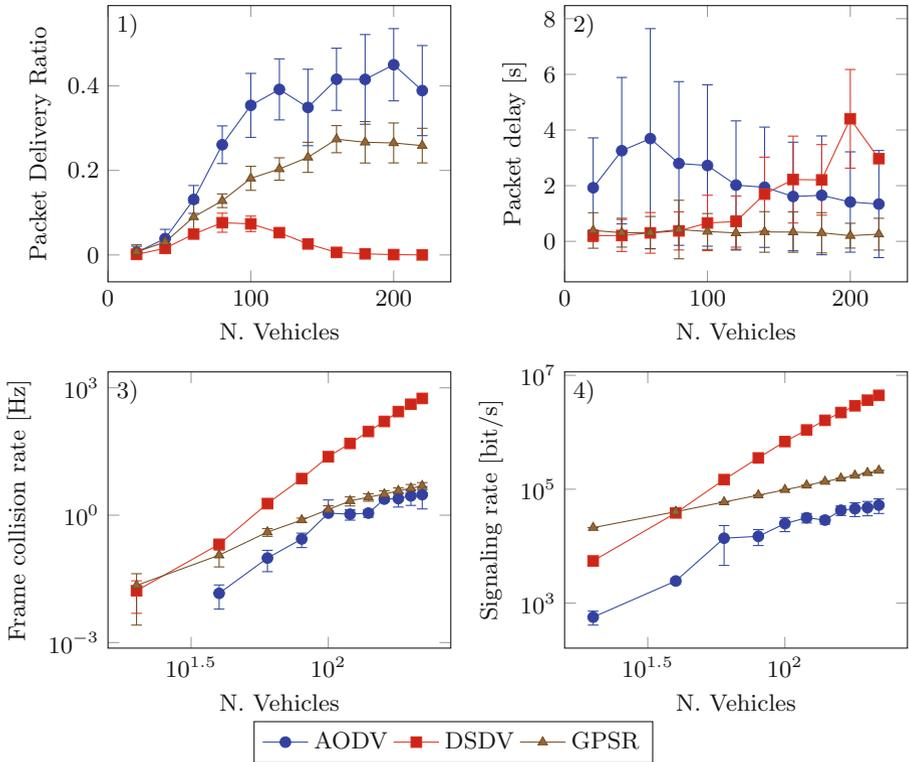
**Fig. 4.** Performances of the selected routing algorithms (AODV, DSDV, and GPSR) for a 300 kbit/s data flow, considering the shadowing effects caused by the buildings.
