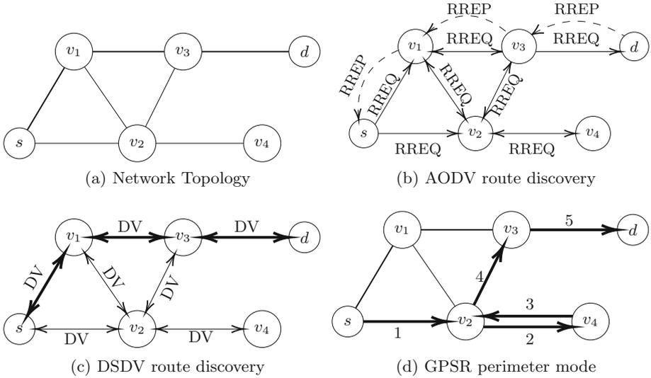
**Fig. 1.** Features of AODV, DSDV, and GPSR. On (a) an example of VANET connectivity graph, with a source vehicle  $s$  and a destination vehicle  $d$ , (b) illustrates the AODV's route discovery process, (c) shows the DSDV's distance vector broadcasting, with the computed route in bold, and (d) shows the route of a packet in GPSR perimeter mode to bypass a void area, where the numbers are the sequence of links on which the data packet is forwarded.
